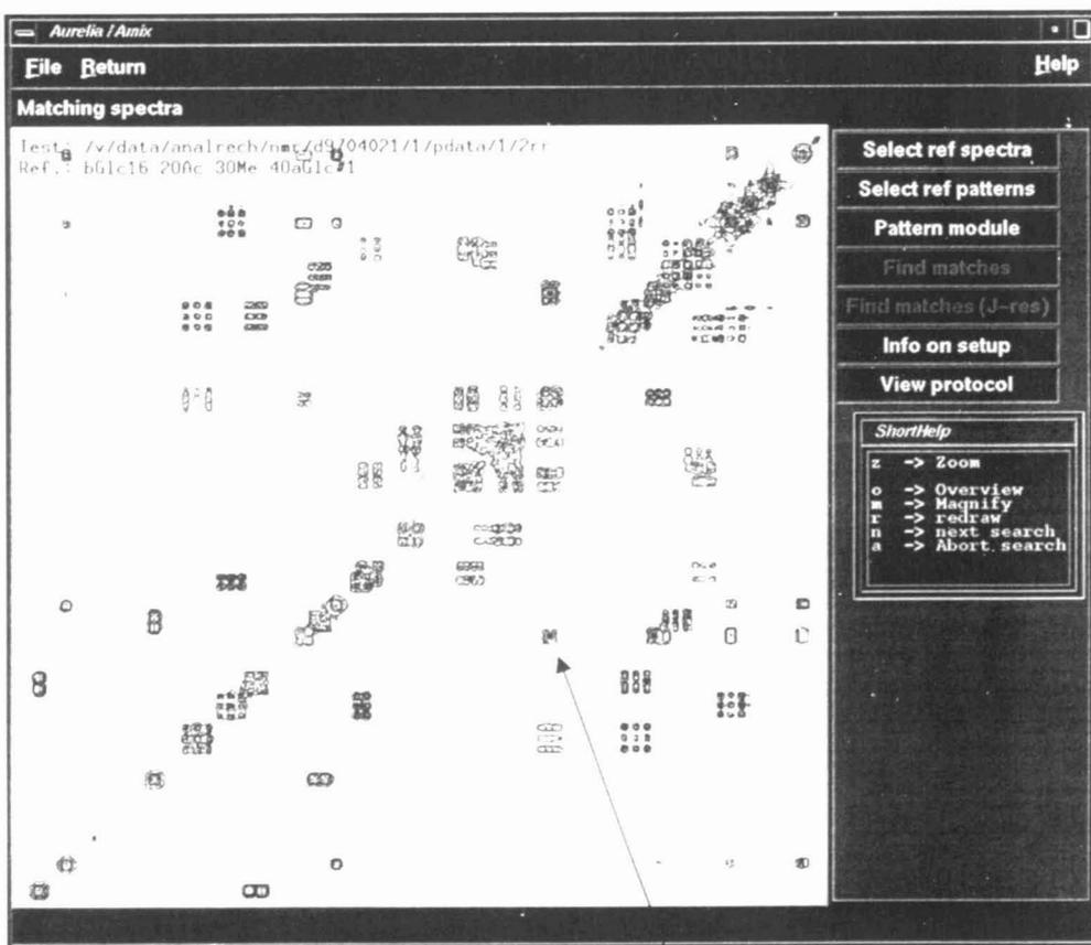
Figure 1: Example of pattern matching with Amix. Each square represents a match between an experimental peak and an entry from the JPD database.
